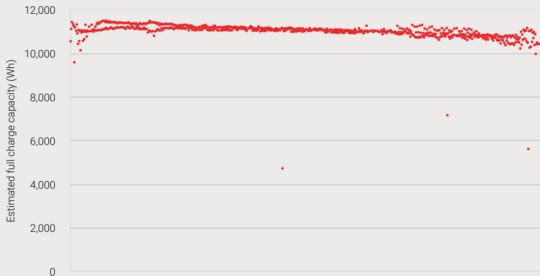
Figure 7: Estimated full charge capacity per cycle by the Redflow battery pack
