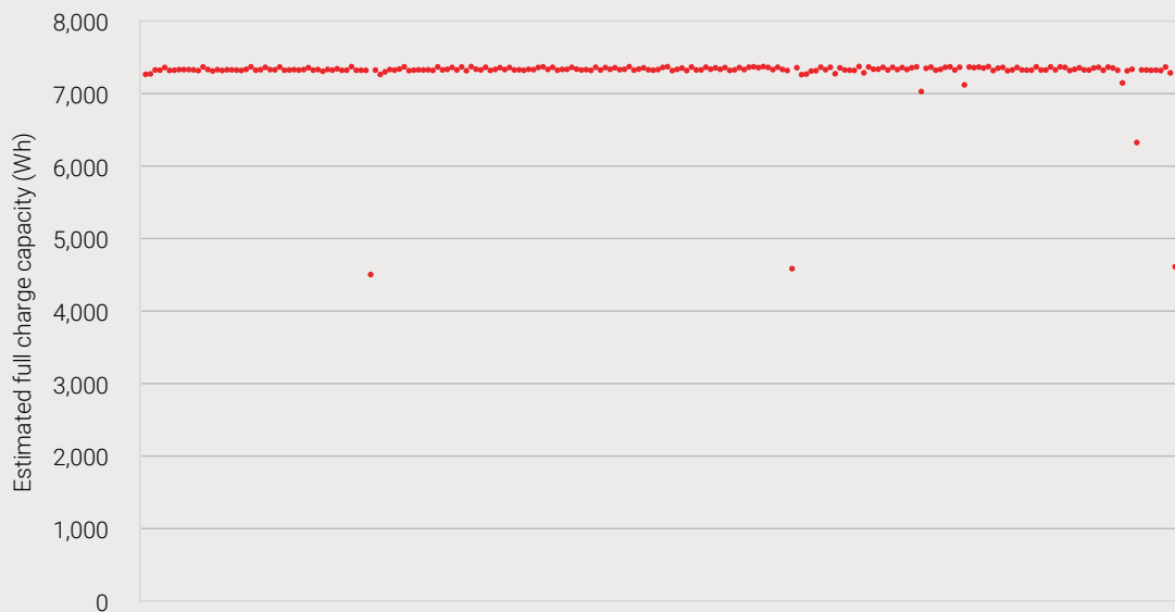
Figure 15: Energy discharged per cycle per cycle by the sonnen battery pack
